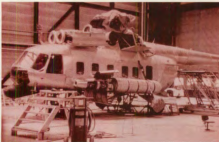
VIP-transport version of Mi-8 Hip-C broken down inside hangar for maintenance. Photo: Courtesy David Isby
